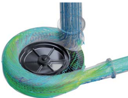
⑤ Air flow on the new side-channel secondary air pump
